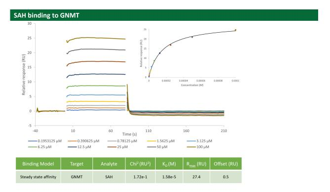
The data were collected on a Biacore 8K using multi-cycle kinetics. The data were analyzed using a steady state affinity model.
