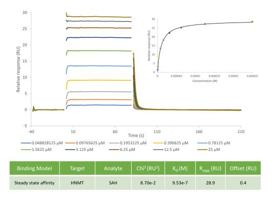
The data were collected on a Biacore 8K using multi-cycle kinetics. The data were analyzed using a steady state affinity model.
