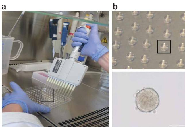
**Figure 2** | Preparation of spheroids. (a) The usage of a multi-micropipette assures consistent and uniform ‘hanging-drops’ throughout a cell culture plate. (b) Magnification of a ‘hanging-drop’ containing a compact and round spheroid, which has been formed within 18 h. Scale bar, 100 μm.
