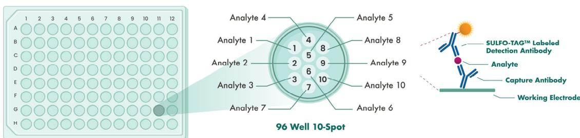
MSD assays at Reaction Biology are performed with 96 well plates containing up to 10 detection spots per well.
