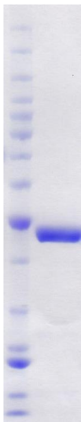
Coomassie blue-stained SDS-PAGE (4-12% acrylamide) of 4 \mu\text{g} of RBC Bcl-2 (GST). MW markers (left) are, from top, 220, 160, 120, 100, 90, 80, 70, 60, 50, 40, 30, 25, 20, 15, 10 kDa.
