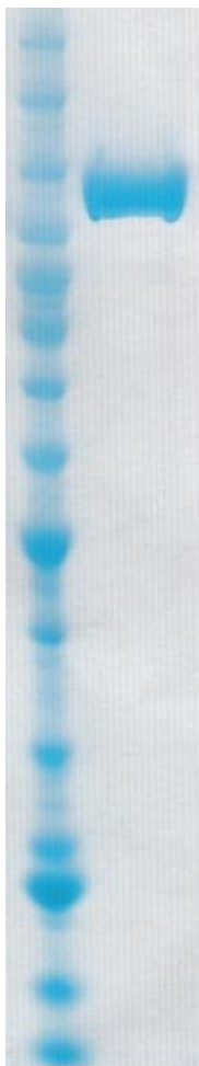
Coomassie blue-stained SDS-PAGE (12% acrylamide) of 2 \mu\text{g} of RBC OGT (His-FLAG). MW markers (left) are, from top, 220, 160, 120, 100, 90, 80, 70, 60, 50 , 40, 30, 25, 20 , 15, 10 kDa.
