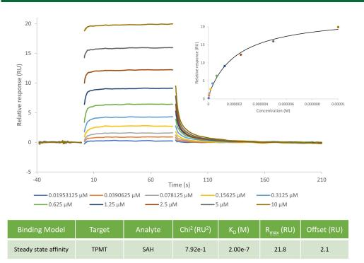
The data were collected on a Biacore 8K using multi-cycle kinetics. The data were analyzed using a steady state affinity model.
