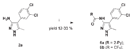
Scheme 2 Synthesis of compounds 6a and 6b. Reaction conditions: i) pyridine-2-carbonyl chloride or trifluoroacetic anhydride, dry pyridine, dry THF, rt, overnight.
